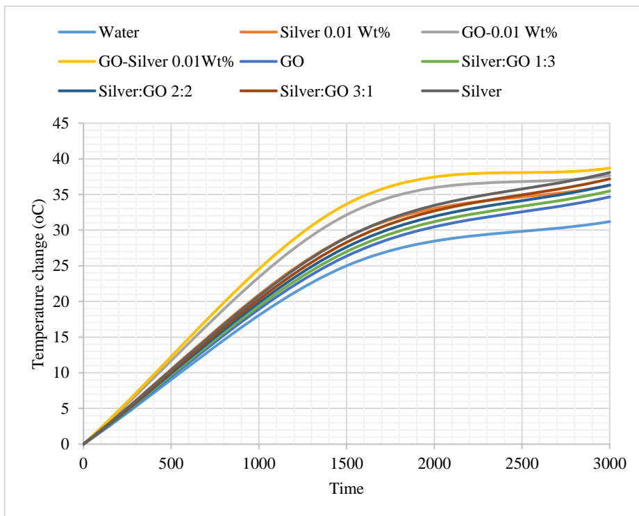
Figure 29. Photothermal experiment results for GOB-silver nanofluids prepared in form Ex-situ using GOB and Ag at a concentration of 0.005 wt%, and In-situ using a concentration of 0.01 wt%
