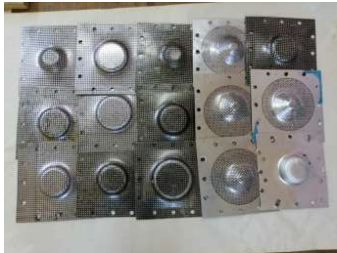
Figure 6. Specimens of formed parts
