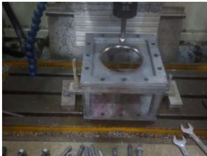
Figure 1. Fixture tools on CNC milling machine
