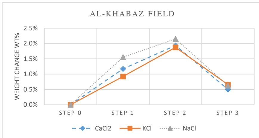
**Figure 2.** Gravimetric test for Al-Khabaz field samples with three solutions; CaCl<sub>2</sub>, KCl, NaCl.
