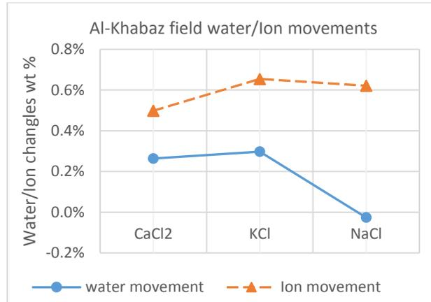
Figure 3. Water and ion movement during the immersion of Al-Khabaz shale samples in three different solutions; CaCl<sub>2</sub>, KCl, and NaCl.
