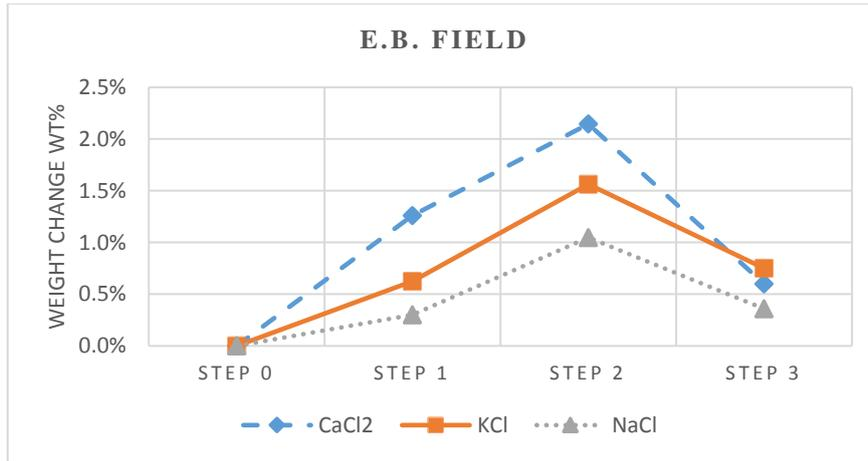
**Figure 1.** Gravimetric test for E.B.field samples in three solutions; CaCl<sub>2</sub>, KCl, NCl.
