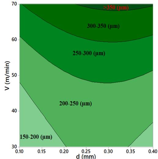
c, Contour Plot of VB vs V, d (Hold f 0.2mm/rev)
