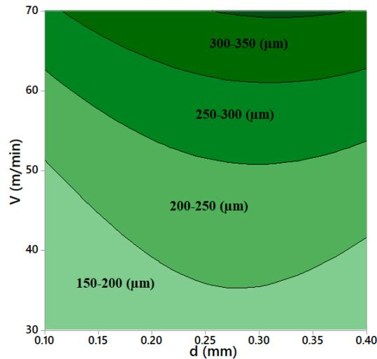
a, Contour Plot of VB vs V, d (Hold f 0.1 mm/rev)
