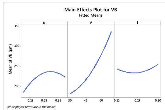
**Figure 4.** Main effects of the cutting parameter on the flank wear
