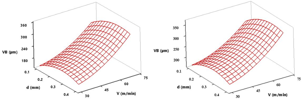
b, Surface Plot of VB vs V, d (Hold f 0.15 mm/rev)      c, Surface Plot of VB vs V, d (Hold f 0.2 mm/rev)
