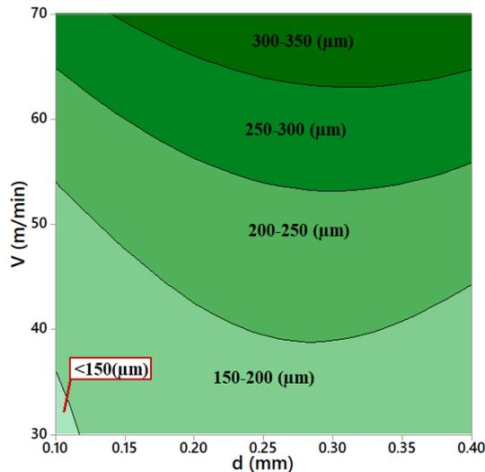
b, Contour Plot of VB vs V, d (Hold f 0.15mm)
