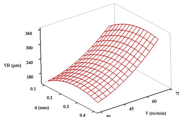
**a, Surface Plot of VB vs V, d (Hold f 0.1mm/rev)**
