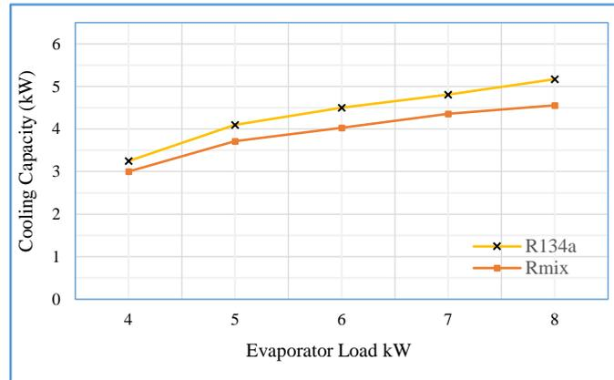
**Figure 10.** Cooling capacity with evaporator load at compressor speed 2300 RPM
