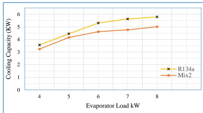
**Figure 9.** Cooling Capacity with Evaporator Load at Compressor Speed 1000 RPM
