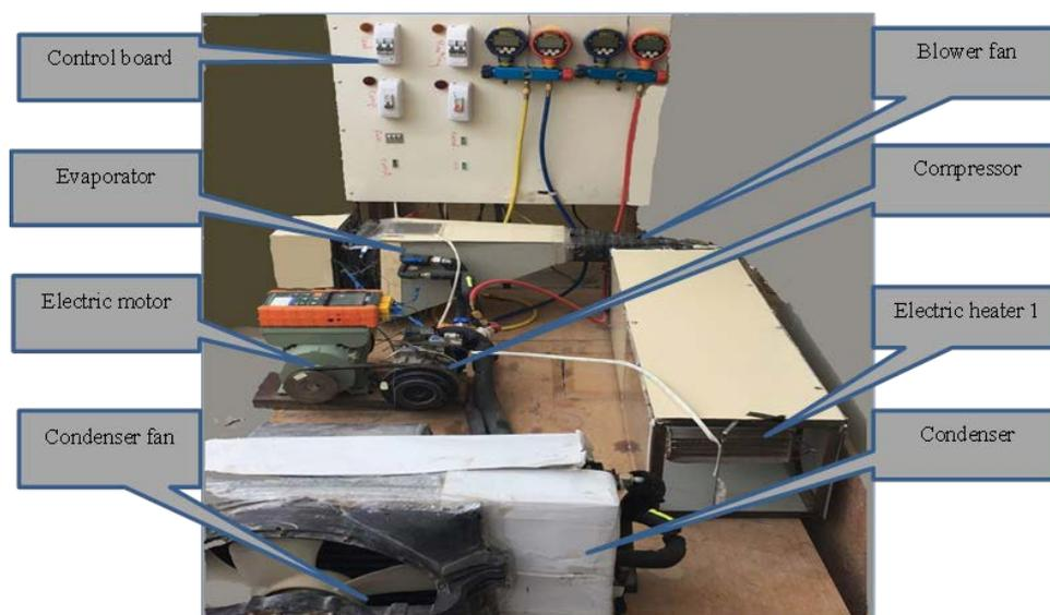
Figure 1. The test Rig
