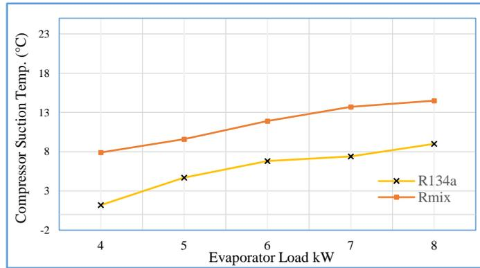
**Figure 5.** Compressor suction temperature with evaporator loads at compressor speed 2300 RPM
