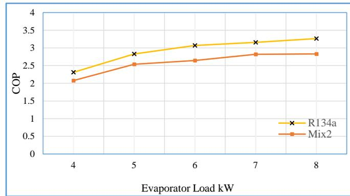
**Figure 13.** Coefficient of performance with evaporator load at compressor speed 1000 RPM
