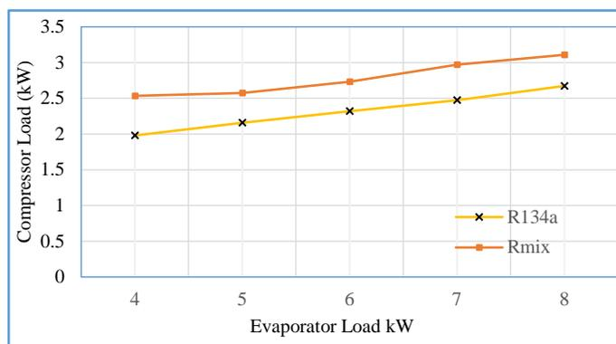
**Figure 12.** Compressor power consumption with evaporator load at compressor speed 2300 RPM
