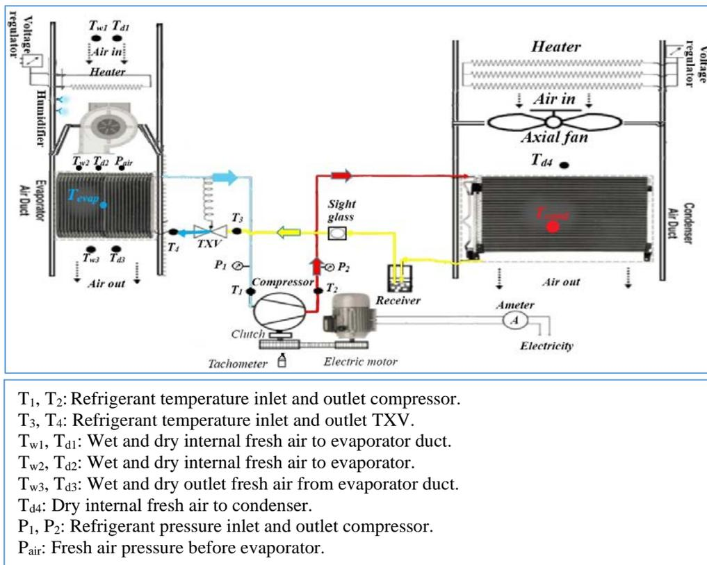
Figure 1. Schematic Diagram of Test Rig
