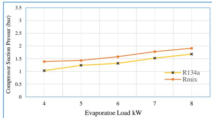
**Figure 6.** Compressor suction pressure with evaporator loads at compressor speed 2300 RPM
