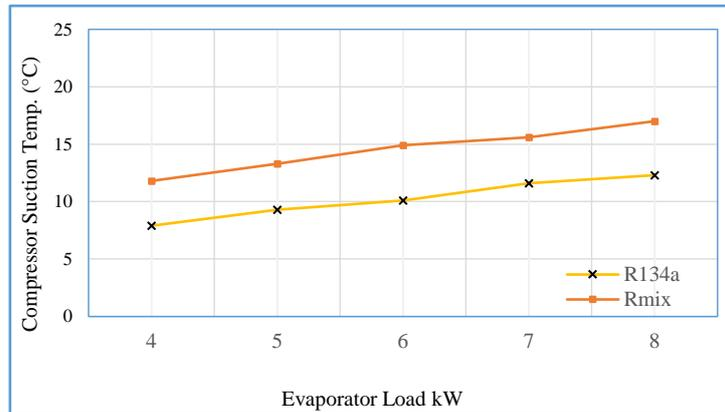
**Figure 3.** Compressor suction temperature with evaporator loads at compressor speed 1000 RPM
