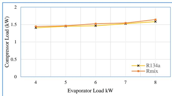
**Figure 11.** Compressor power consumption with evaporator load at compressor speed 1000 RPM
