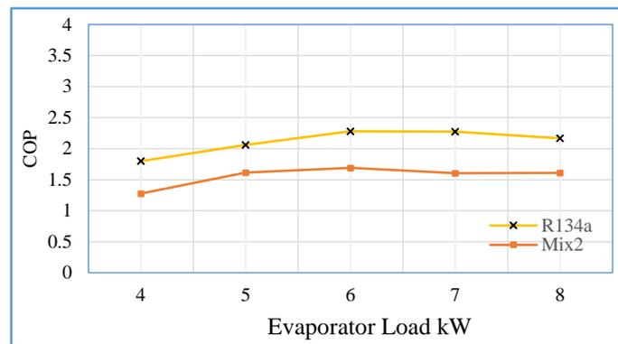
**Figure 14.** Coefficient of performance with evaporator load at compressor speed 2300 RPM
