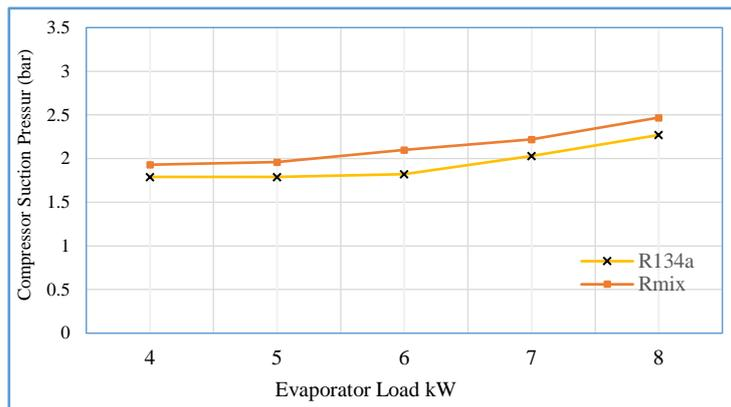
**Figure 4.** Compressor suction pressure with evaporator loads at compressor speed 1000 RPM
