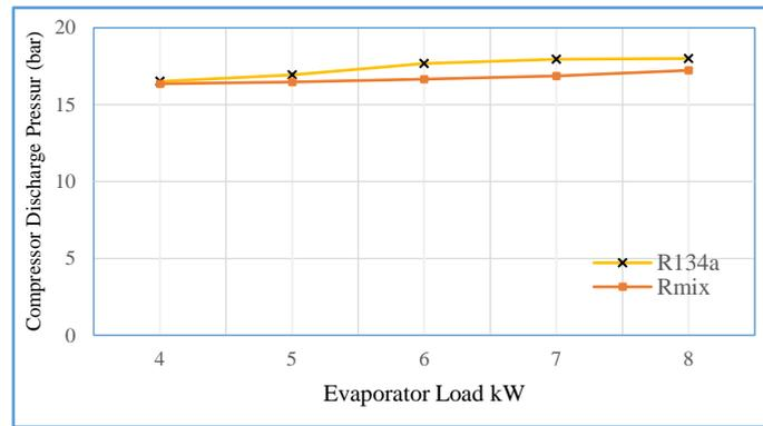
**Figure 8.** Compressor discharge pressure with evaporator load at compressor speed at 1000 RPM
