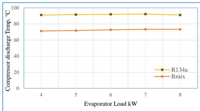
**Figure 7.** Compressor Discharge Temp. with Evaporator Load at Compressor Speed 1000 RPM
