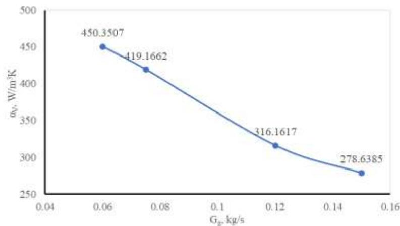
**Figure 5.** Effect of initial air mass flow rate on volumetric heat transfer coefficient ( $T_g = 180^\circ\text{C}$ )
