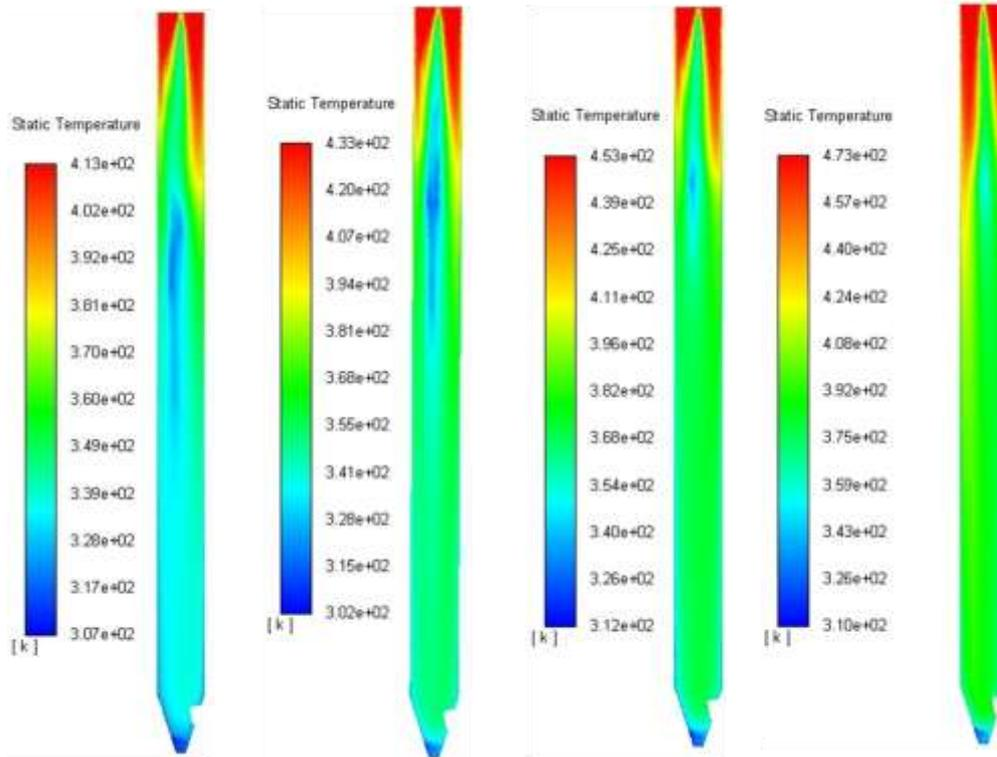
**Figure 2.** Changes in air temperature profile along the spray tower obtained from CFD simulations for the initial air mass flow rate  $G_g = 0.075$  kg/s.
