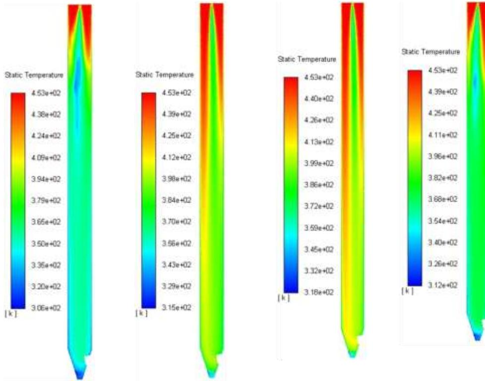
**Figure 4.** Changes in air temperature profile along the spray tower obtained from CFD simulations for the initial air temperature  $T_g = 180$  °C.
