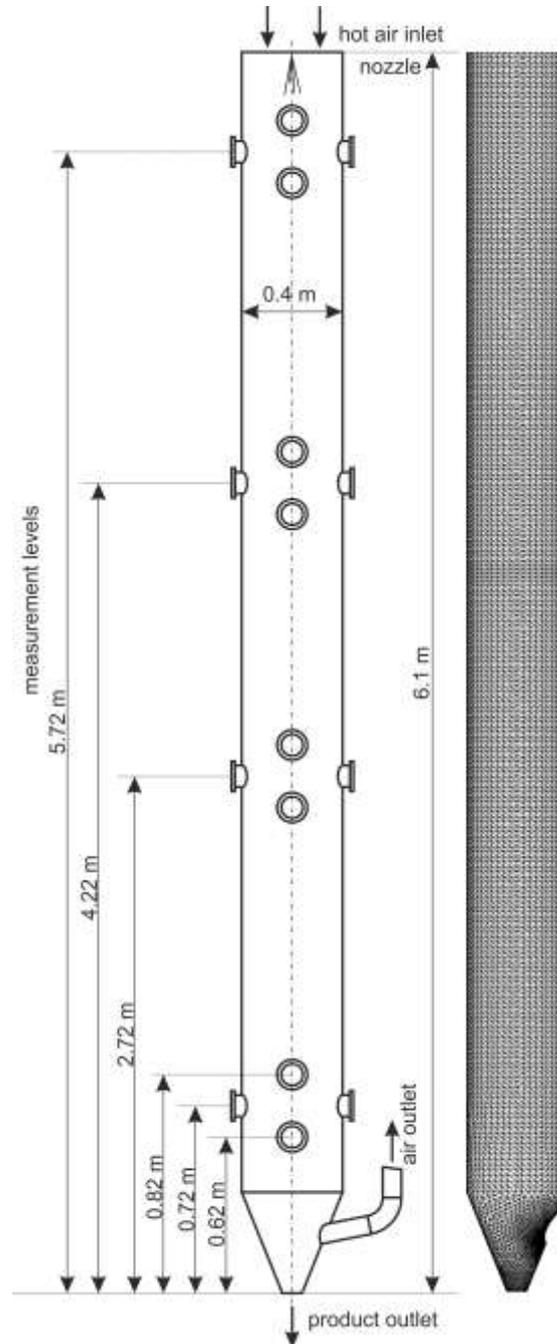
Figure 1. Geometry of spray dryer [3]
