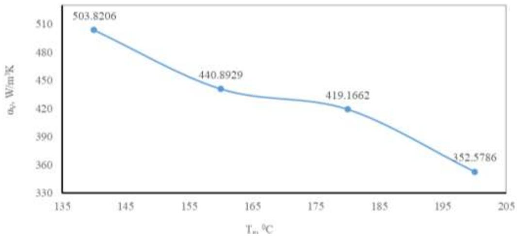
**Figure 3.** Change of volumetric heat transfer at various inlet air temperature ( $G_g = 0.075$  kg/s)
