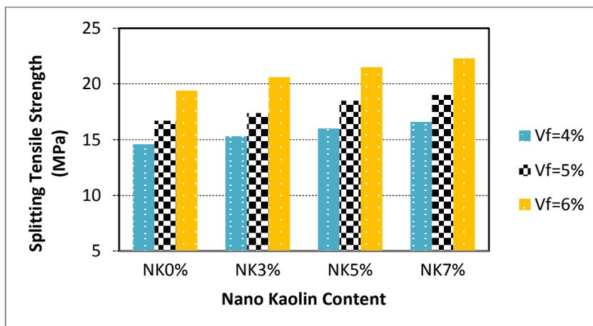
**Figure 3.** Comparison of the Splitting tensile strength of SIFCON with different Nano Kaolin Content
