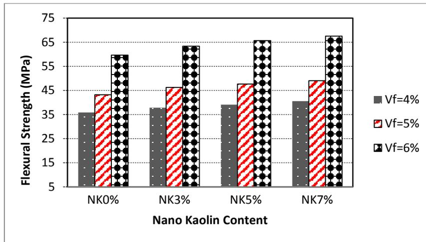
Figure 4. Comparison of the Modulus of Rupture strength of SIFCON with different Nano Kaolin Content
