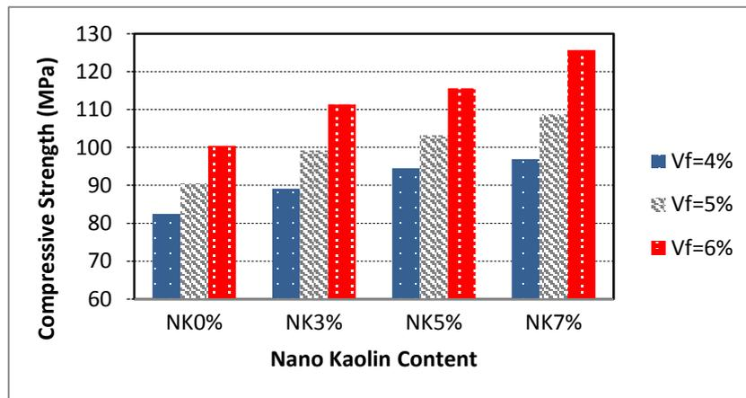
**Figure 2.** Comparison of the compressive strength of SIFCON with different Nano Kaolin Content
