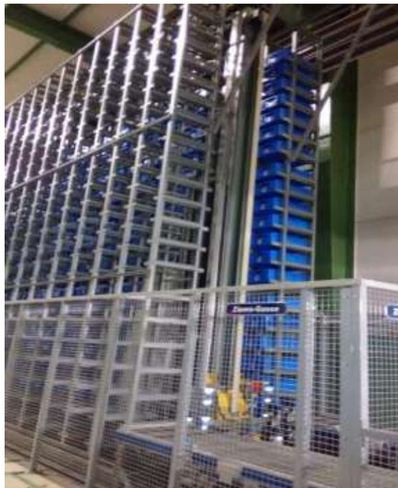
**Figure 1.** Automatic small parts warehouse (ASPW) at the Institute (ILM).
