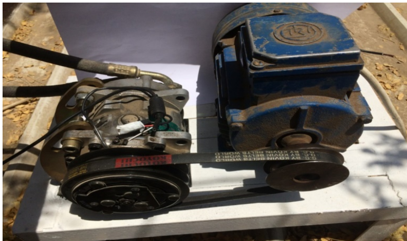
Figure 4. Variable speed compressor and motor system
