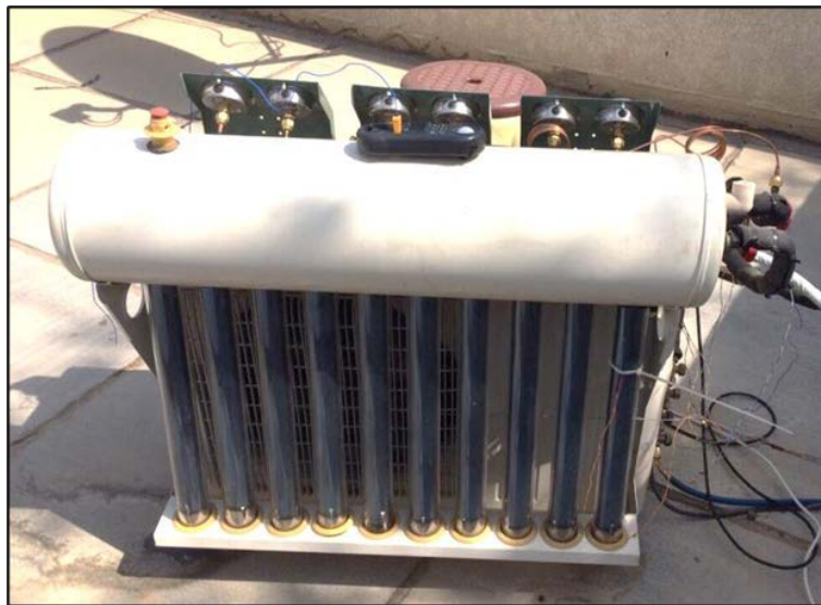
Figure 6. Solar collector assisted air conditioner
