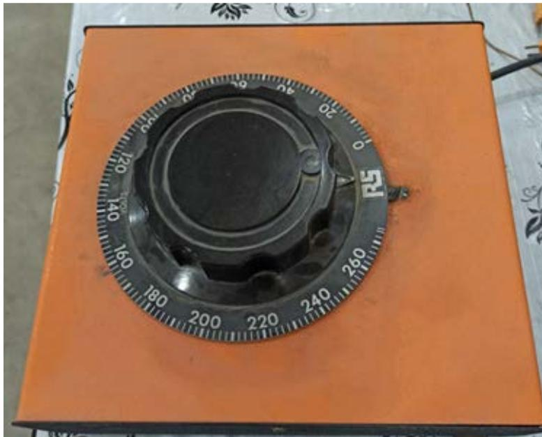
**Figure 4.** Photograph of Voltage Variation Device
