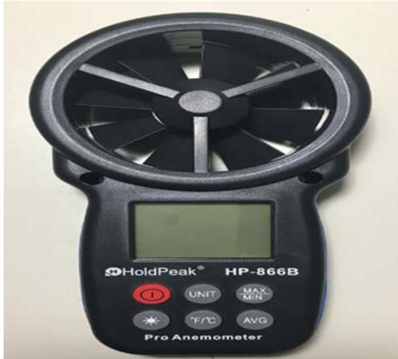
**Figure 3.** Hand-held digital anemometer
