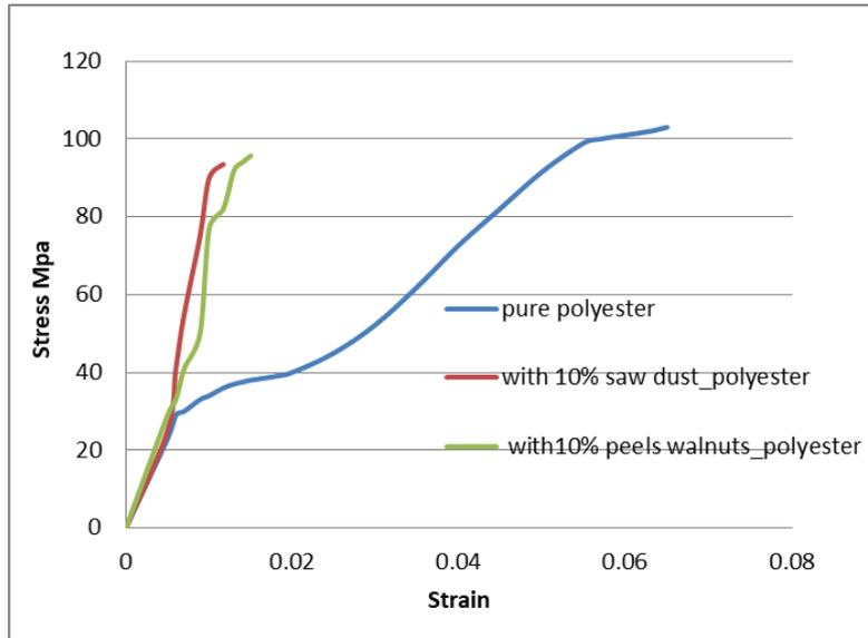
Figure 7. Stress – strain curve for compression test for 10 % from 4.75 mm particles mixed in polyester
