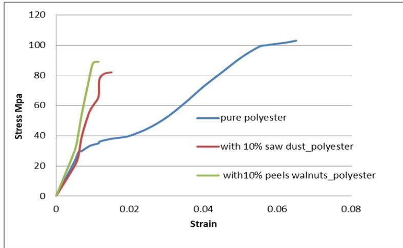
Figure 10. Stress – strain curve for compression test for 10% from 9.5 mm particles mixed in polyester
