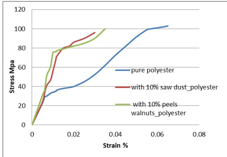
Figure 4. Stress – strain curve for compression test for 10 % from 2.36mm particles mixed in polyester
