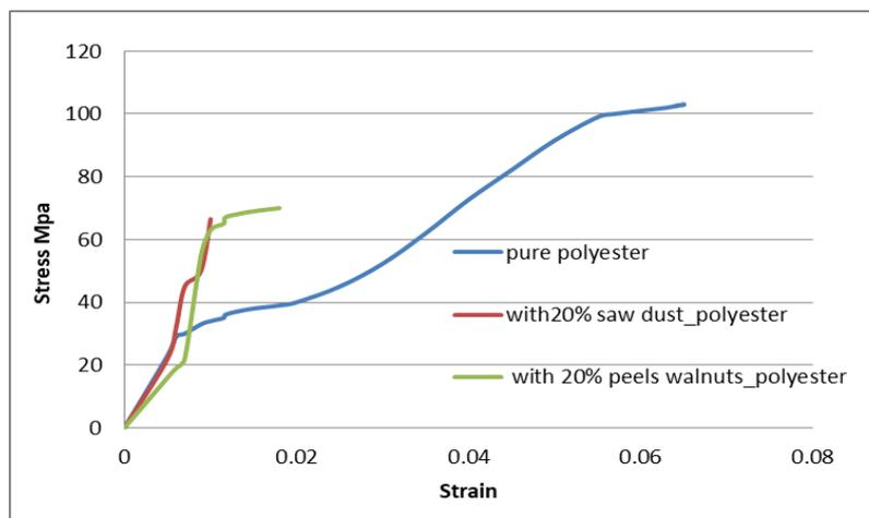
Figure 9. Stress – strain curve for compression test for 20% from 4.75 mm particles mixed in polyester
