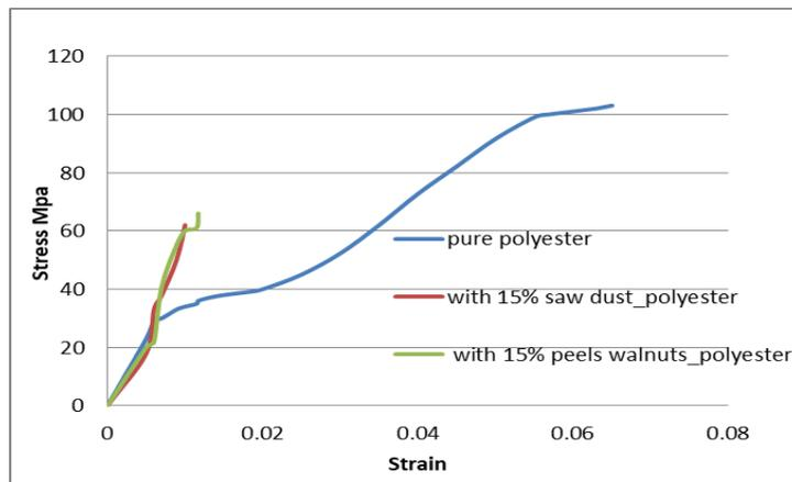
Figure 11. Stress – strain curve for compression test for 15% from 9.5 mm particles mixed in polyester
