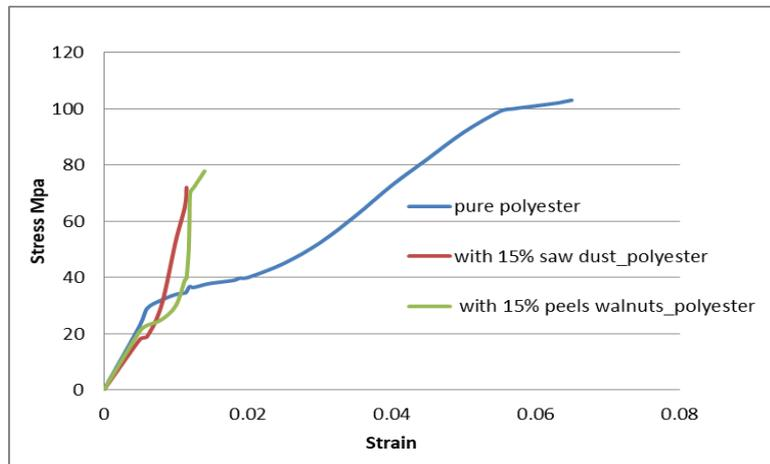
Figure 8. Stress – strain curve for compression test for 15 % from 4.75 mm particles mixed in polyester
