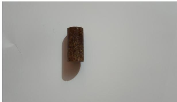
**Figure 2.** The test specimens of polyester mixing with particles
