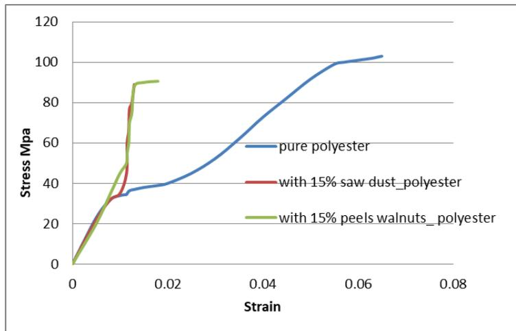
Figure 5. Stress – strain curve for compression test for 15 % from 2.36mm particles mixed in polyester
