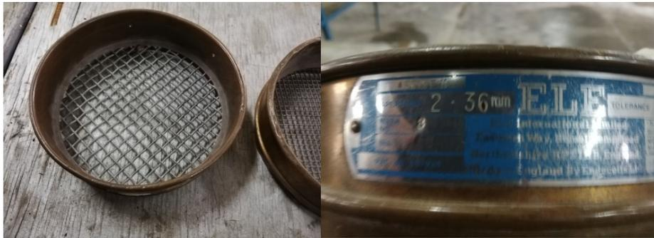
**Figure 1.** Sieves to isolate the particles
