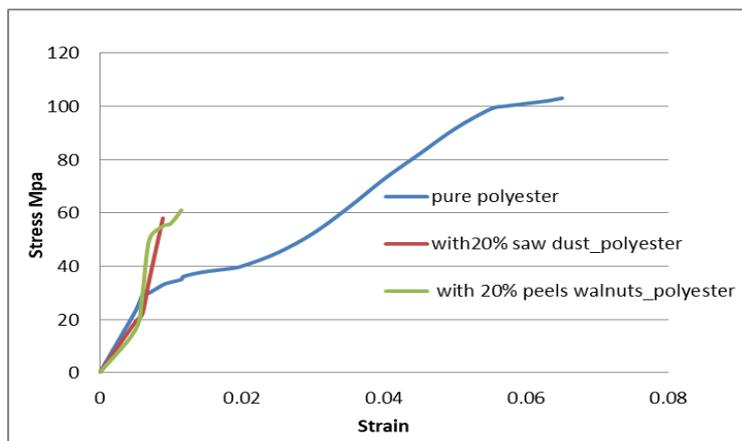
Figure 12. Stress – strain curve for compression test for 20% from 9.5 mm particles mixed in polyester
