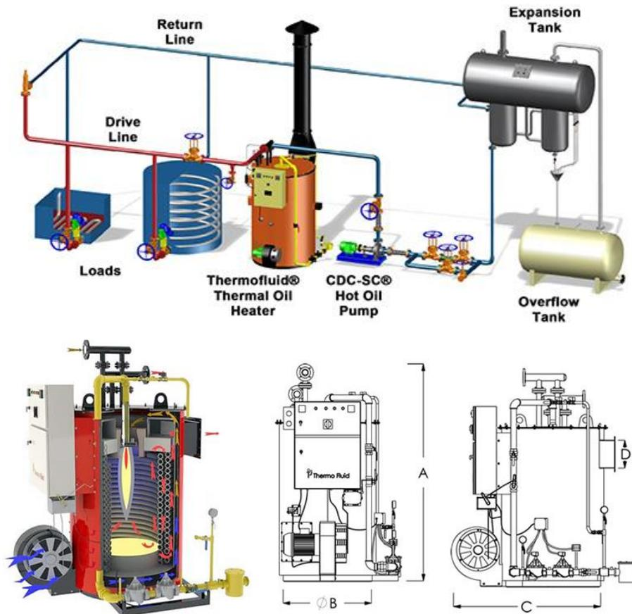
**Figure 2.** A typical thermal oil system is fitted on the tanker to heat cargo oil
