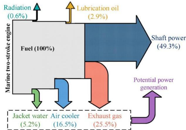
**Figure 1.** Scheme of thermal balance for a marine diesel engine by MAN 12K98ME / MC [37]
