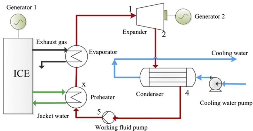
**Figure 4.** Configuration of ORC waste heat recovery system from exhaust gas cooled water
