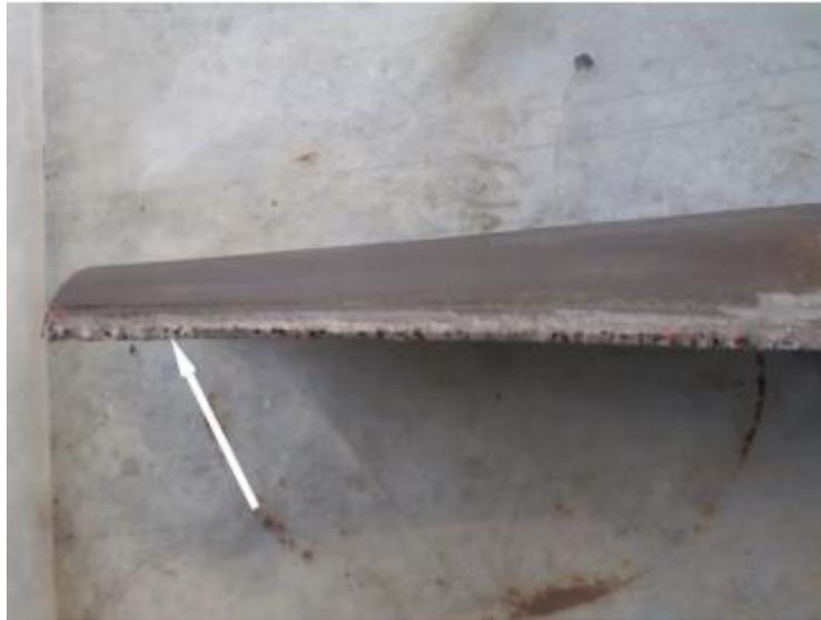
**Figure 3.** Erosion of the leading edge of steam turbine blade
