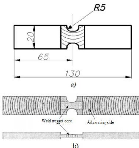
Fig. 2. (a) Sample for determining the tensile strength of the weld metal at FSW and (b) the scheme of cutting out the sample to determine the tensile strength of the weld nugget core
