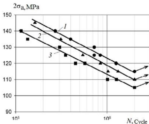
**Figure 4.** (1) Curves of fatigue of the base material and (2) welded joints obtained by FSW and (3) arc welding with non-consumable electrode.
