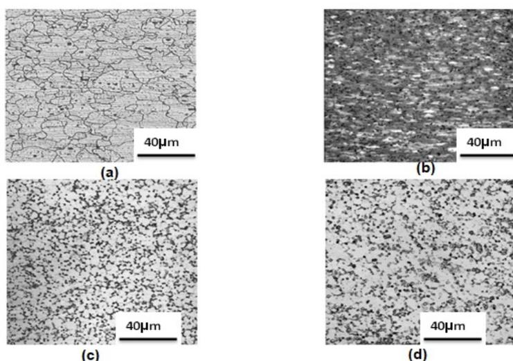
**Figure 3.** Microstructure of sheets of (a) AZ31B alloys, (b) 7075 alloys, (c) the core of the weld seam of AZ31B and 7075 (d) alloys with a thickness of 5 mm
