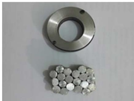
**Figure 1.** Pin and disc specimens.
