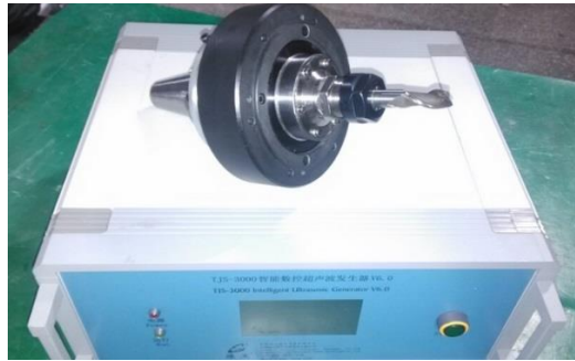
Figure 2. Ultrasonic tool holder and its ultrasonic generator.
