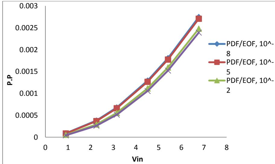
**Figure 10.** Variation of pumping power (watt) with velocity inlet of pressure driven.
