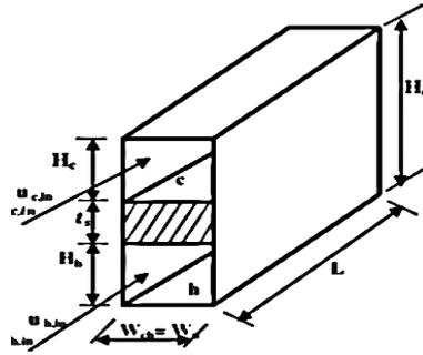
**Figure 2.** A unit of heat exchanger consists of hot and cold channels at parallel flow [8].
