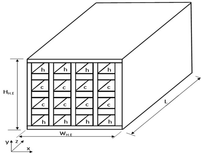
**Figure 1.** Schematic model of the microchannel heat exchanger.
