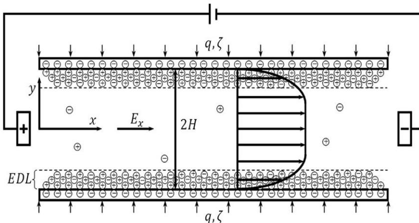
**Figure 3.** Scheme formed of electric double layer on surface wall [10]
