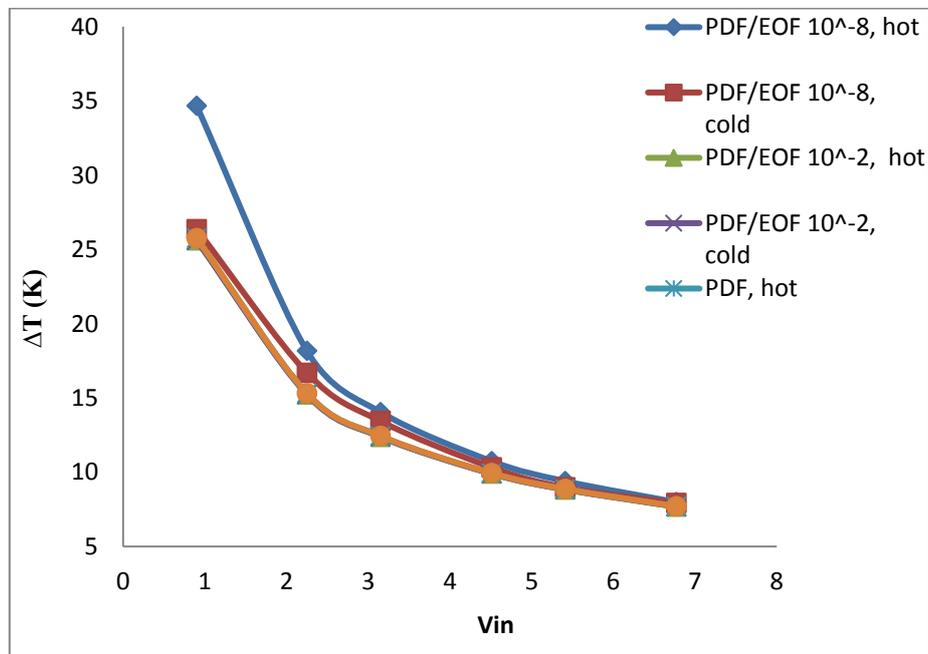
**Figure 11.** Comparisons between temperature differences for a hot and cold channel with velocity inlet.
