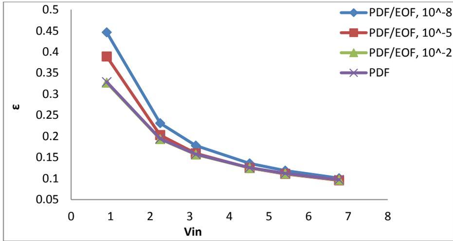
Figure 7. Variation of effectiveness with velocity inlet of pressure driven.
