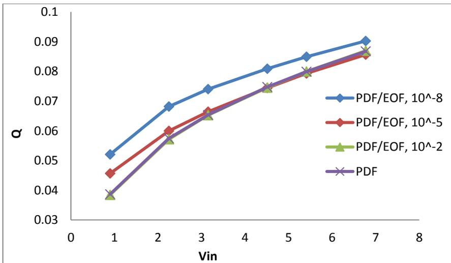
Figure 9. Variation of heat transfer (watt) with velocity inlet of pressure driven .
