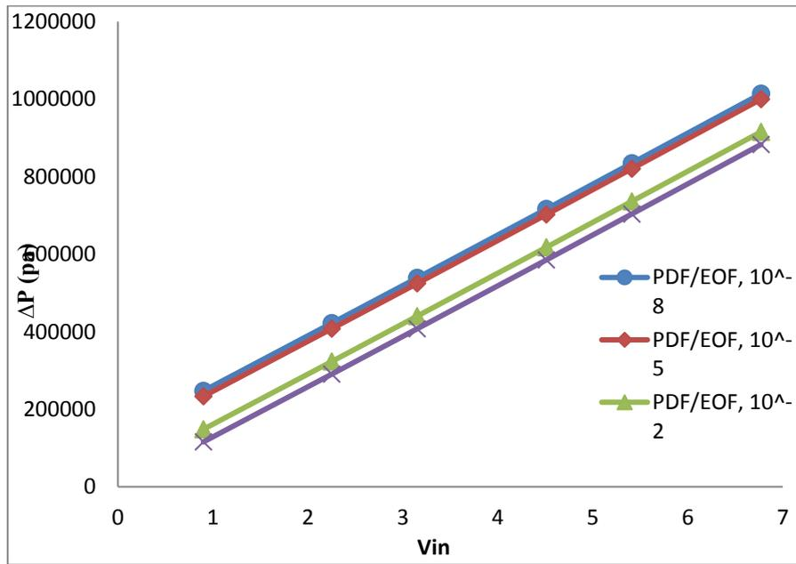
Figure 5. Variation of total pressure drop (pa) with velocity inlet of pressure driven.
