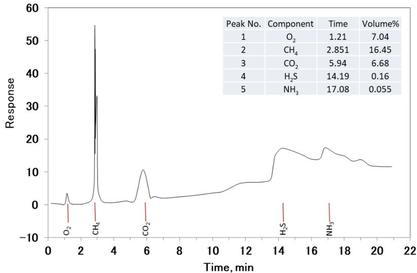
**Figure 2.** GC analysis of the produced biogas
