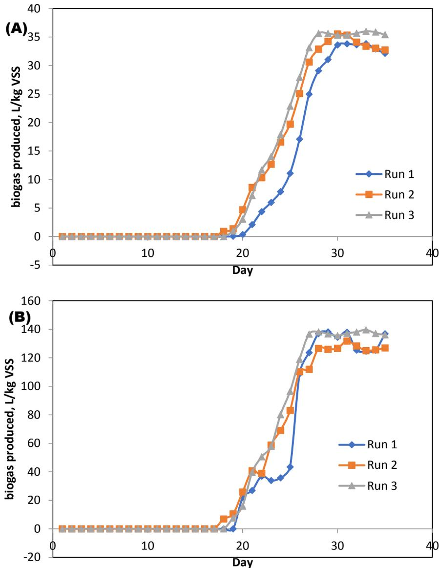
**Figure 3.** Profile of (A) commutative gas production rate vs. time for lab scale (25L) unit (B) cumulative gas production rate vs. time for pilot unit (1000L)
