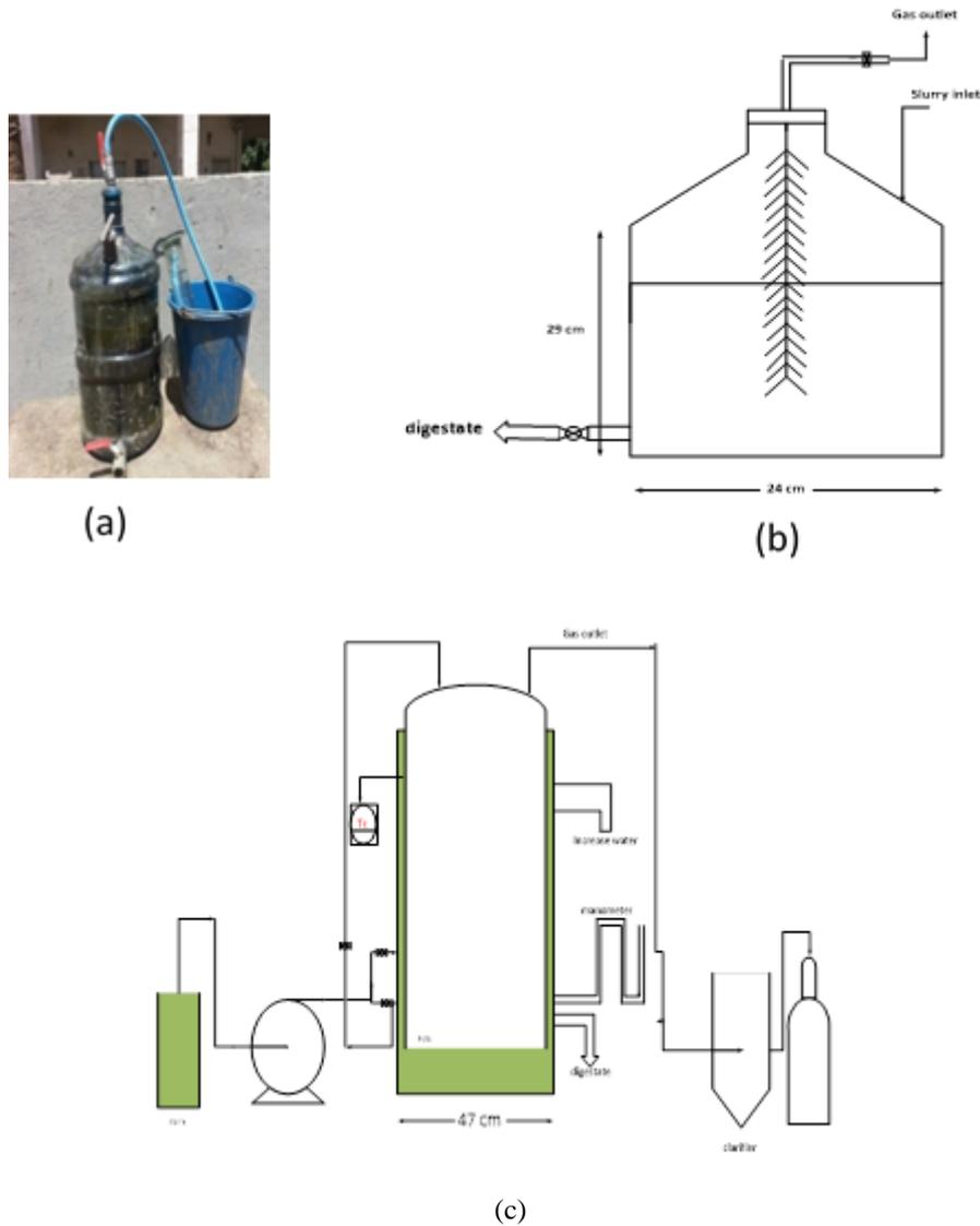
**Figure 1.** Photo and schematic diagram for the used digester, (a, b) the lab scale digester V= 25 L, (c) the pilot scale unit used V= 1000 L.
