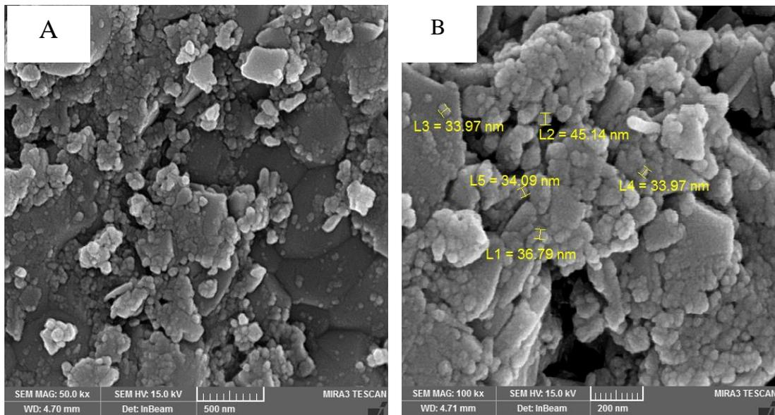
**Figure 3.** FE-SEM images of 0 mol% ZnO at 1100 °C of compacted bioceramic samples at different magnifications.
