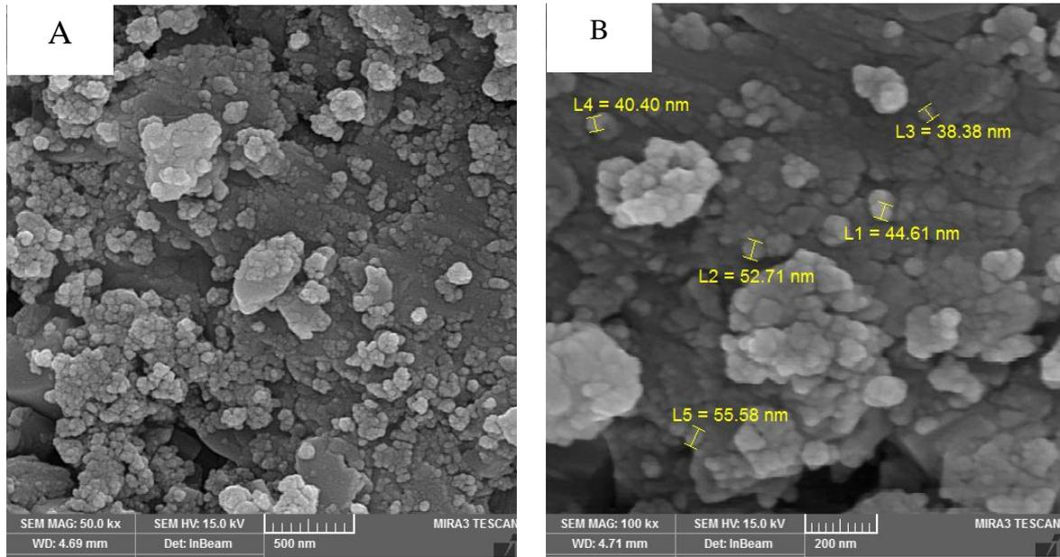
**Figure 4.** FE-SEM of 8 mol% ZnO at 1100 °C of compacted samples at different magnifications.
