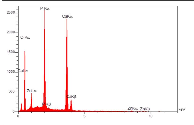
**Figure 6.** EDS results at 8 mol% ZnO of compacted bioceramics samples at 1100 °C.
