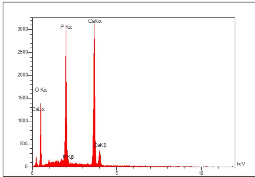
**Figure 5.** EDS results at 0 mol % ZnO of compacted bioceramics samples at 1100 °C.
