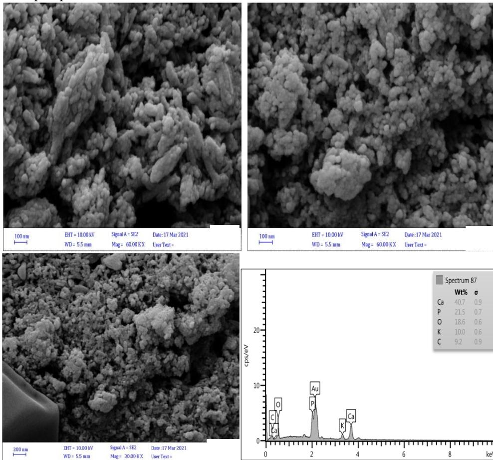
**Figure 7.** FE-SEM and EDS results of 8 mol% ZnO compacted sample at different magnifications after immersion in SBF for 14 days.
