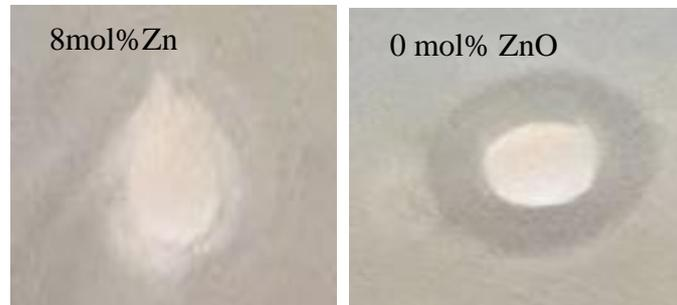
**Figure 8.** Antibacterial activity of (0, and 8) mol% of ZnO co-doped specimens against *E. Coli* bacteria.
