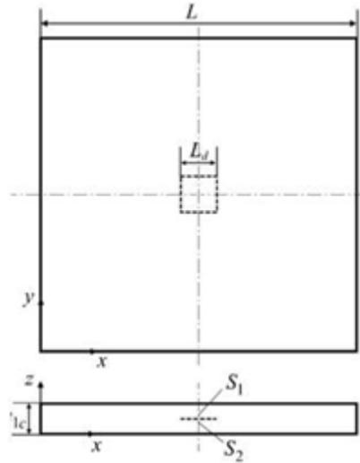
**Figure 4.** Defective Plate
