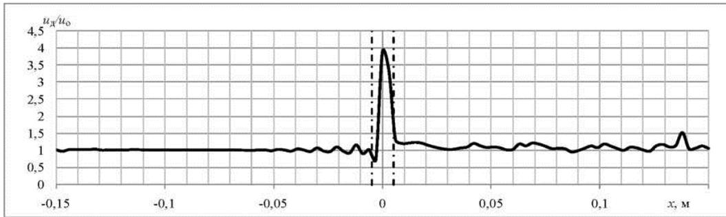
**Figure 11.** Graph of the ratio of the component displacements  $U_z$  in a plate with delamination to the corresponding component in a defect-free plate
