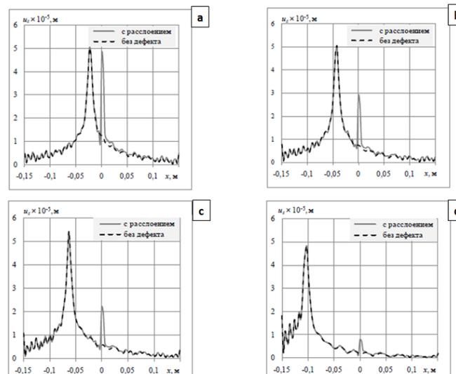
**Figure 9.** The distribution along the line passing through the center of the delamination, the amplitudes of displacements for different relative to the geometric center of the plate the positions of the point of application of an external periodic effect, mm: 23 (a); 43 (b); 63 (c); 103 (d)
