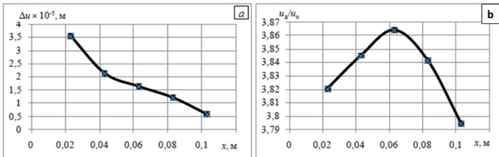
**Figure 12.** Change of the difference (a) and the ratio of displacements (b) in the defective and defect-free plates depending on the distance of the point of application of an external periodic effect from the center of the defect
