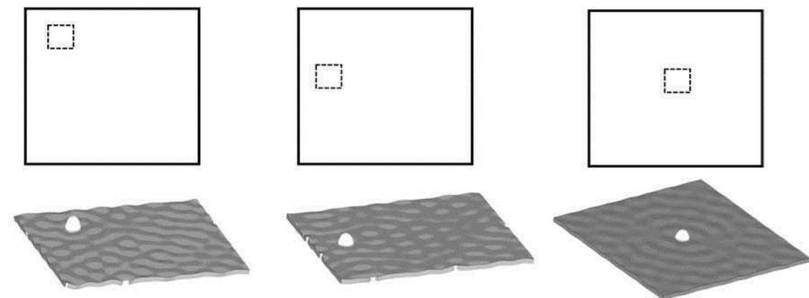
**Figure 6.** Own vibration shapes at different layering locations on the plate
