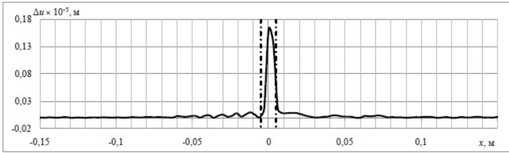
**Figure 10.** Graph of the difference of the displacement component  $U_z$  in a plate with a delamination and in a defect-free plate
