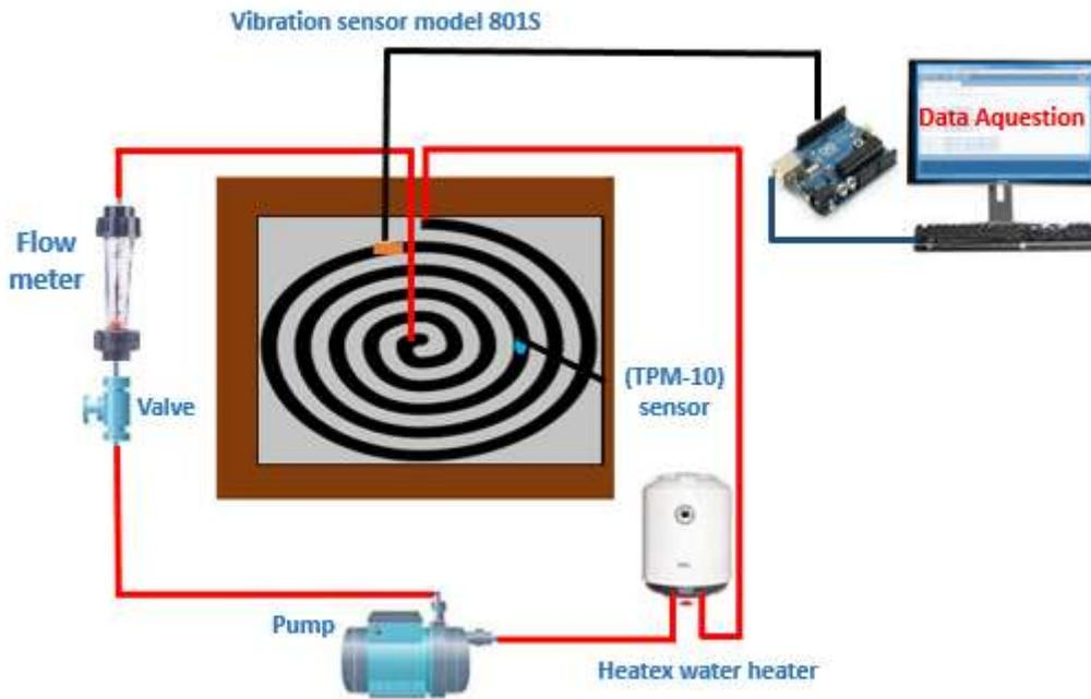
**Figure 2.** Schematic diagram of vibration experimental.
