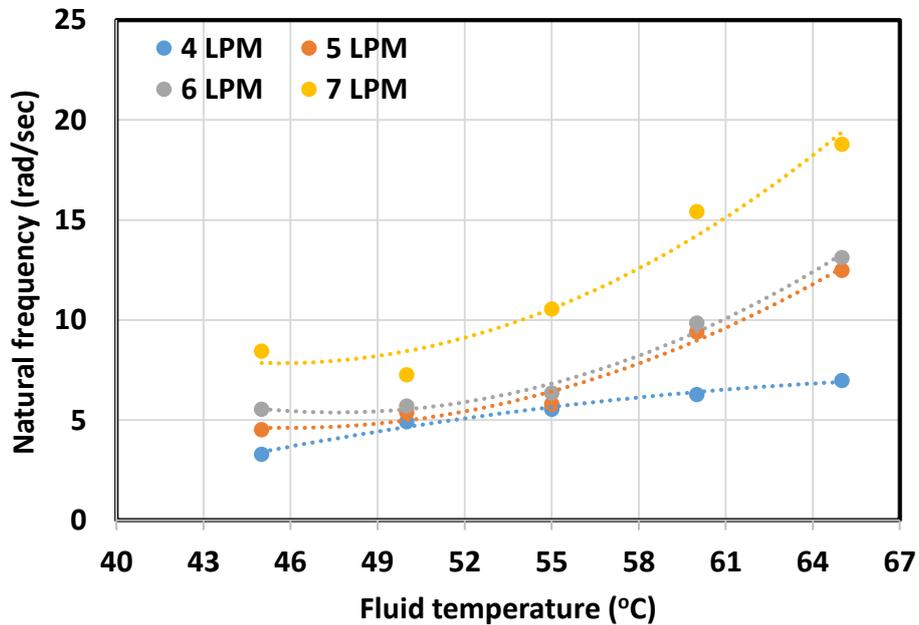
Figure 4. Show the relation between fluid temperature versus natural frequency.
