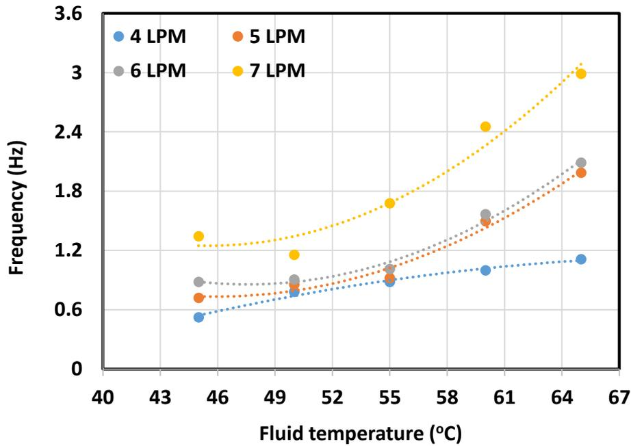
Figure 3. Show the variation of fluid temperature in frequency.
