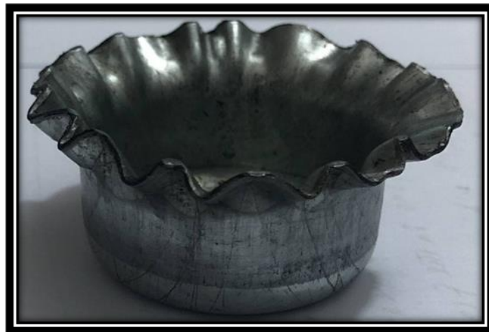
Figure 5. The wrinkling defect in state two.
