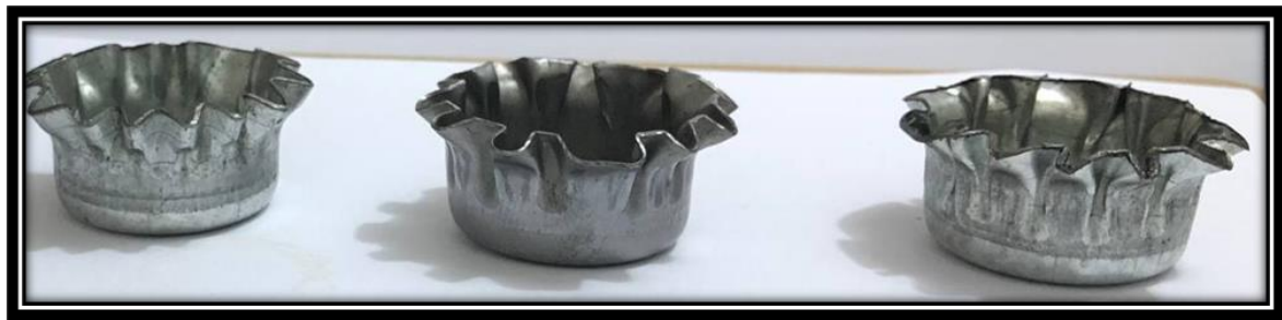
Figure 3. The wrinkling defect in the product
