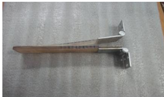
Figure 20. Failed DCB Sample
