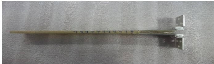
Figure 5. Fracture toughness specimen- A DCB specimen
