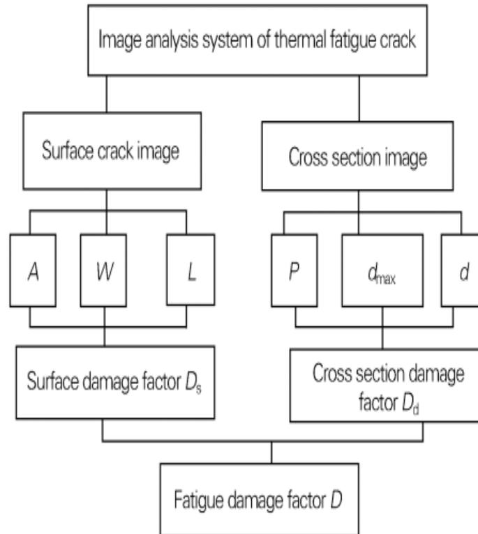
**Figure 1.** Flow chart of thermal fatigue crack analysis system [24]
