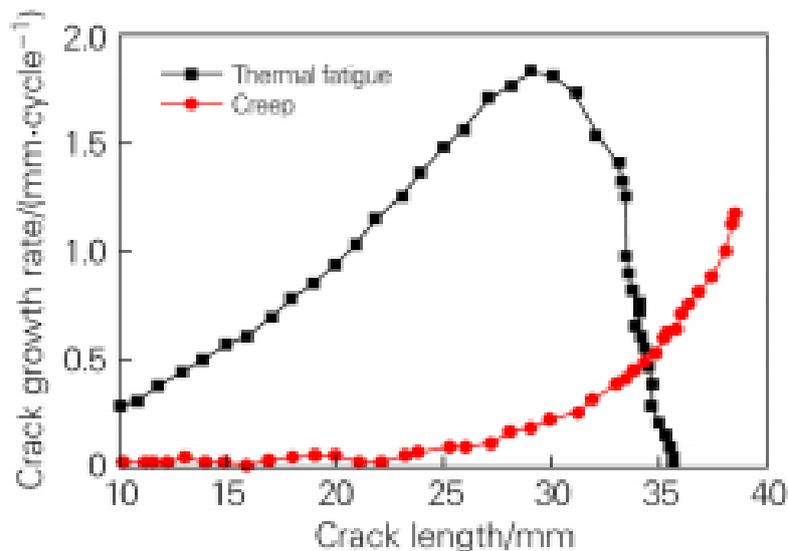
**Figure 5.** Crack growth rate of H13 steel under creep and thermal fatigue
