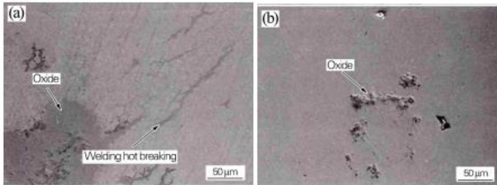
Figure 2. Surface morphology of H13 steel (a) and Co-based alloy coating (b) after 1000 thermal cycles
