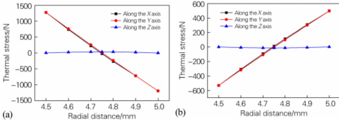
**Figure 4.** Thermal stress along radial distance of the H13 hot work die steel during TF cycle (a) during heating; (b) during cooling.
