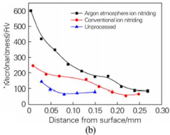
Figure 3. Hardness gradient of H13 hot work die steel without thermal fatigue cycle (a) and after 3000 thermal fatigue cycle (b) [18]
