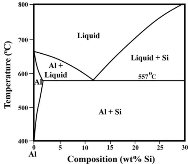
Figure 2. The Al-Si phase diagram [24]
