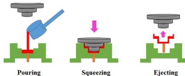
**Figure 6.** The diagram of the squeeze casting technique [76]
