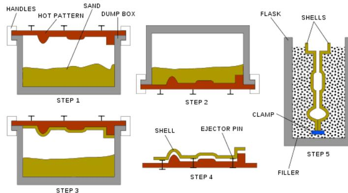
**Figure 3.** The production process of shell mold casting [51]
