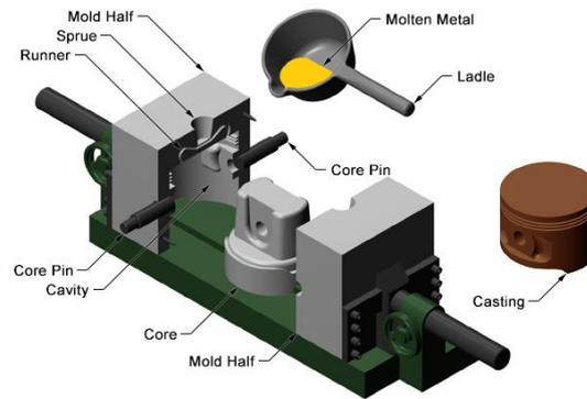
**Figure 5.** The permanent mold casting process for automotive aluminum alloy piston [66]
