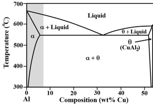
**Figure 1.** The general Al-Cu phase diagram [19]
