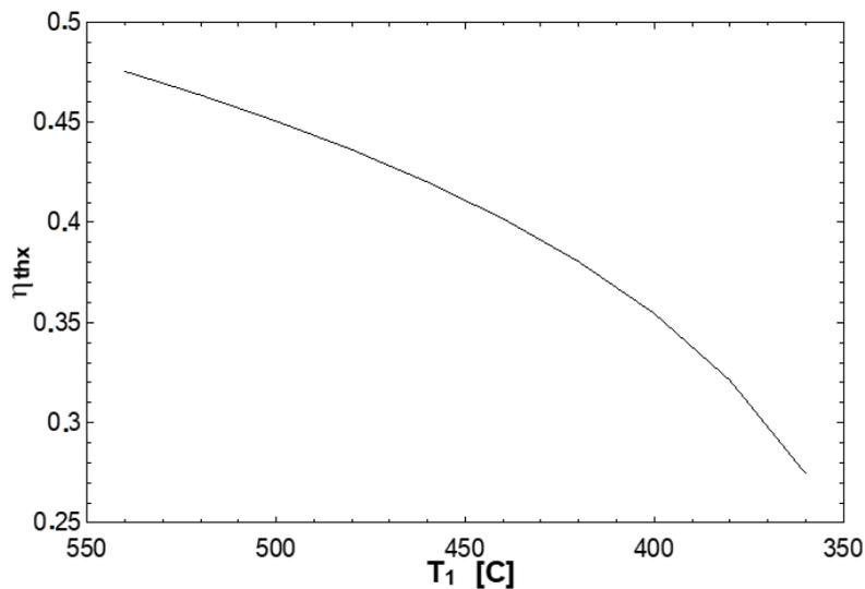
Figure 3. The effect of turbine inlet temperature on the thermal efficiency of the power plant.
