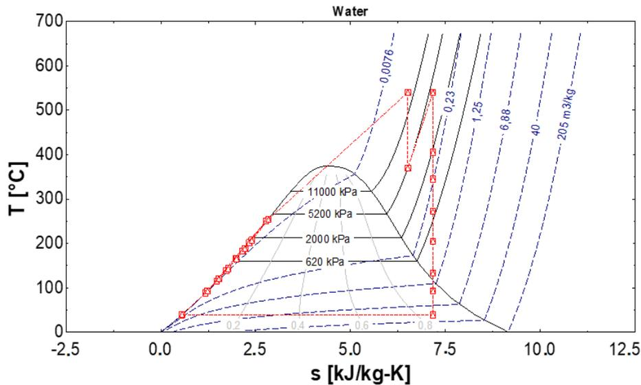
Figure 2. Temperatures and Entropies in T\_S diagram of the Reheat Rankin cycle.
