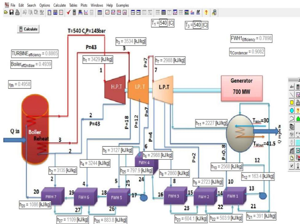
Figure 1. Process flow diagram of the considered power plant
