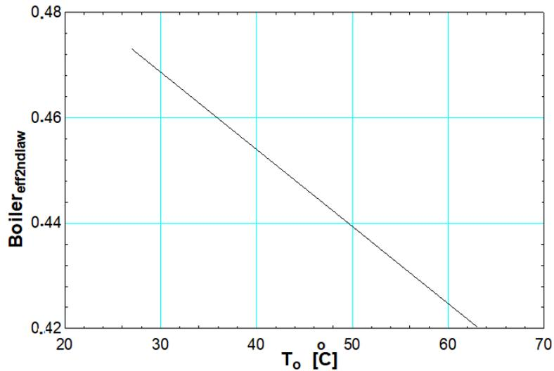
**Figure 4.** Shows the ambient temperature effect on the thermal Boiler’s efficiency.
