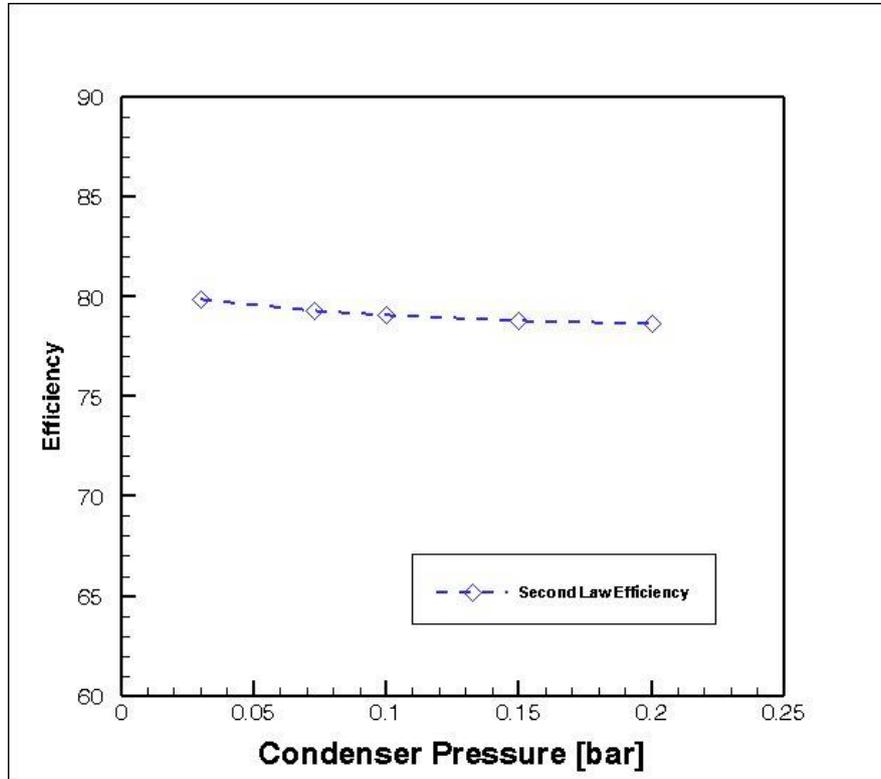
Figure 6. The effect of condenser pressure on the exergy efficiency of the cycle
