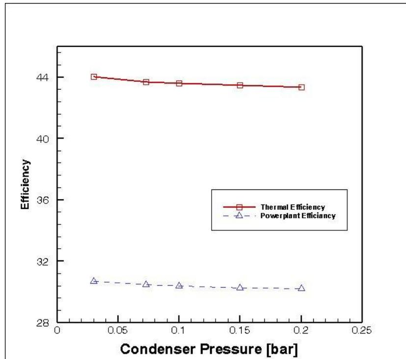
**Figure 5.** The effect of condenser pressure on thermal efficiencies of the cycle and powerplant
