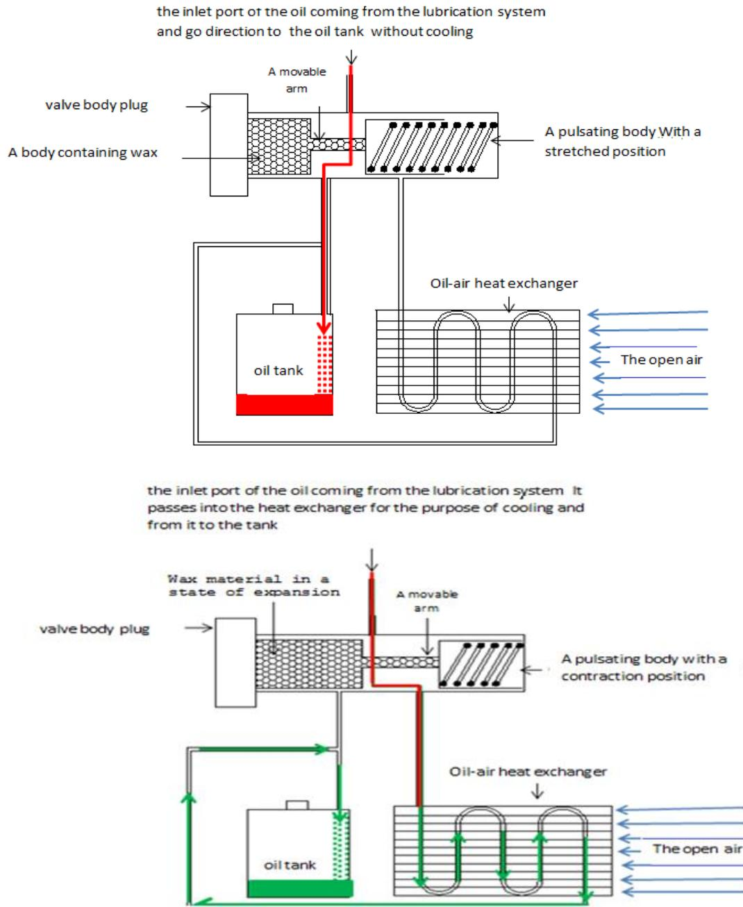
**Figure 2.** Principle operation of origin thermostat
