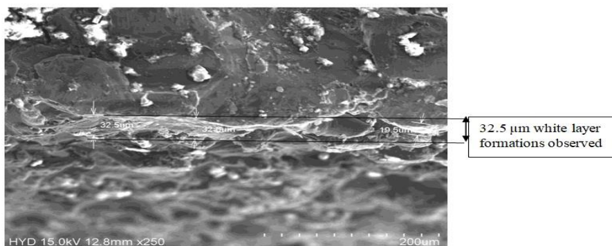
Figure 11. The morphology of Al6061 with SiC after EDM process (10 A, T on 75 \mu sec, T off 80 \mu sec) White layer (32.4 \mu m) at X250.
