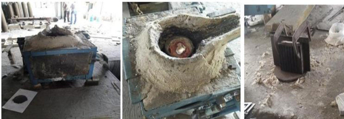
Figure 2. Furnace and Cast Iron Die, liquid aluminum metal matrix pouring in to cast iron die.
