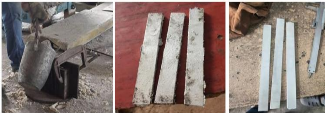
Figure 3. Aluminum 6061 with SiC Work pieces and after machining of stir casted Aluminum 6061 with SiC
