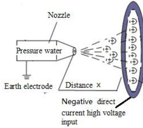
**Figure 2.** rinciple of spray induction charging.
