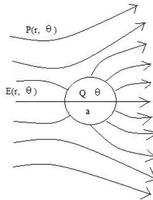
Figure 4. Charged dielectric sphere in uniform electric field.
