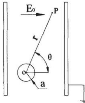
Figure 3. Dielectric sphere in an uniform electric field.
