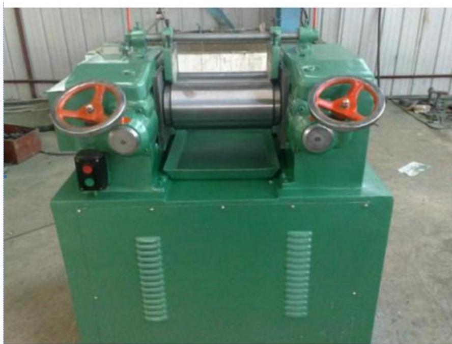
**Figure 1.** XK-160 open mill.
