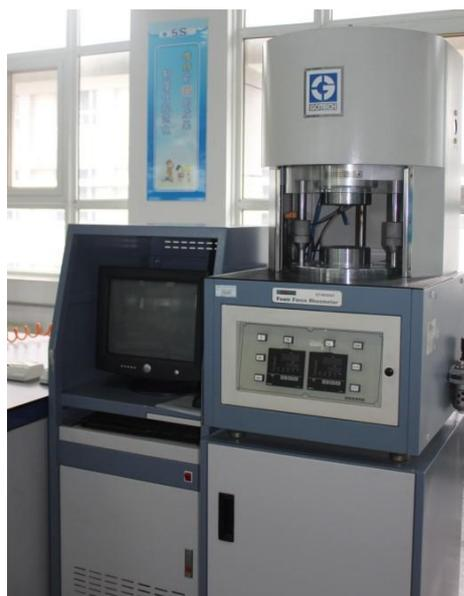
**Figure 2.** GT-M2000 curometer.
