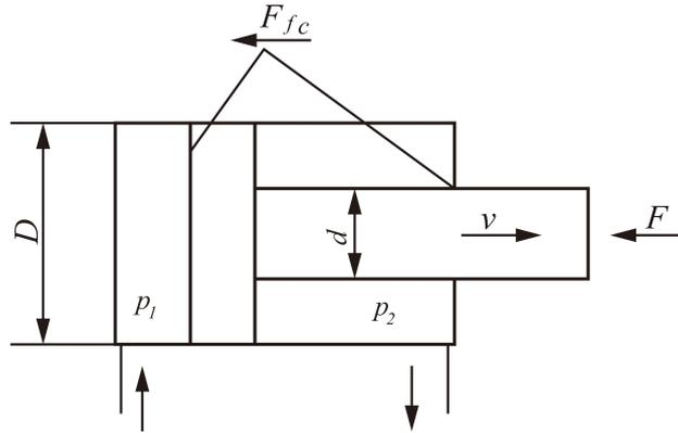
Figure 2. Hydraulic cylinder schematic diagram.
