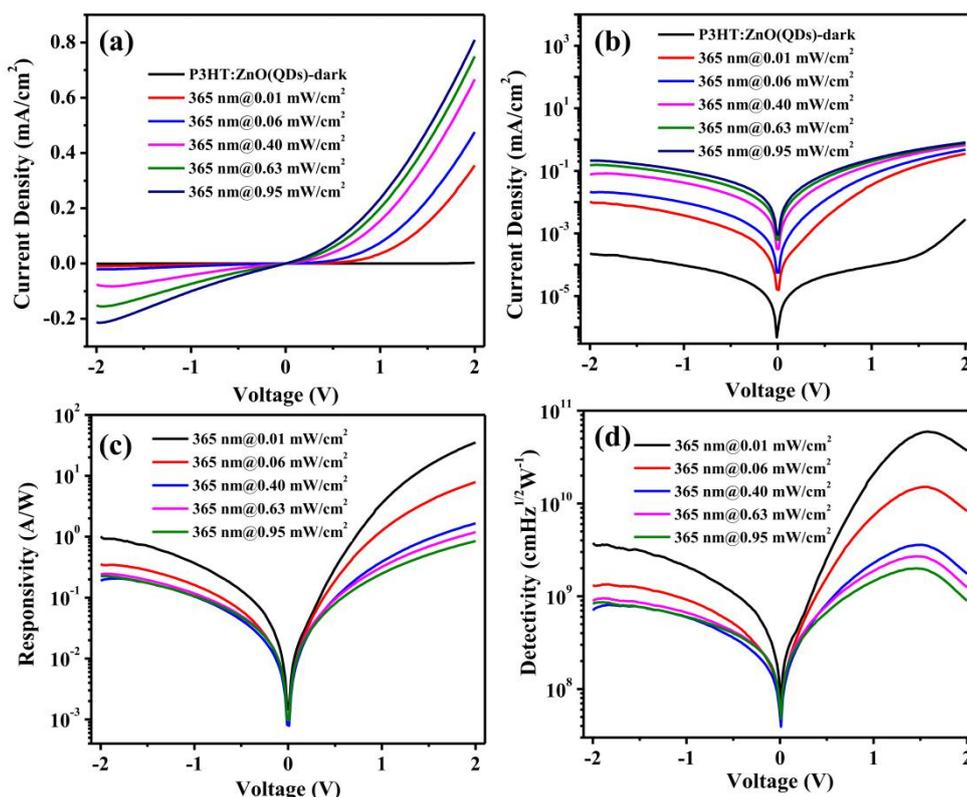
**Figure 4.** (a) The J-V curves and (b) the log J vis-à-vis V curves for the ZQDs based detector under different light illuminations; (c) the relationship between the responsivity (R) and the bias voltage and (d) the relationship between the detectivity and the bias voltage for the P3HT based detector with different illumination intensity ( $\lambda=365$  nm).
