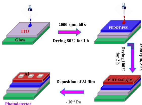
**Figure 1.** The schematic illustration of the fabrication process for the P3HT/ZQDs UV detector.
