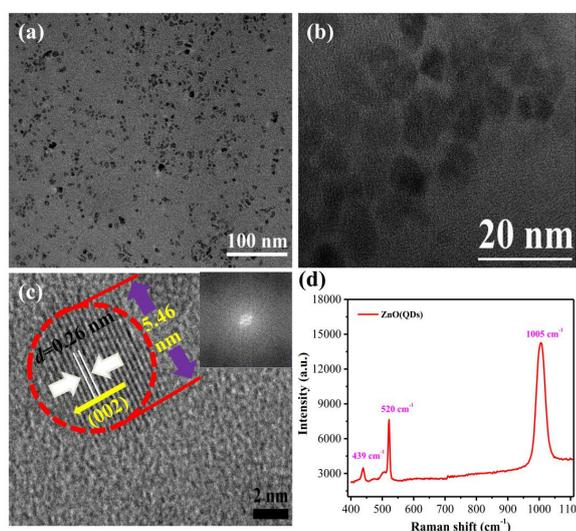
**Figure 2.** (a) and (b)TEM image of ZQDs; (c) A typical single ZQDs, the lattice fringe spacing is 0.26 nm; (d) Raman spectrum of ZQDs.
