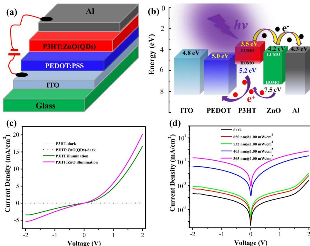
**Figure 3.** (a) Schematic and (b) energy level diagram of a ITO/PEDOT:PSS/P3HT:ZnO(QDs)/Al photovoltaic detector; (c) J-V characteristic curves of the photovoltaic detector using P3HT or P3HT: ZQDs as the active layer illuminated with fluorescent lamp ( $1.7 \text{ mW}/\text{cm}^2$ ); (d) Plot of log current density as functions of voltage for the P3HT: ZQDs detector under different light illuminations.
